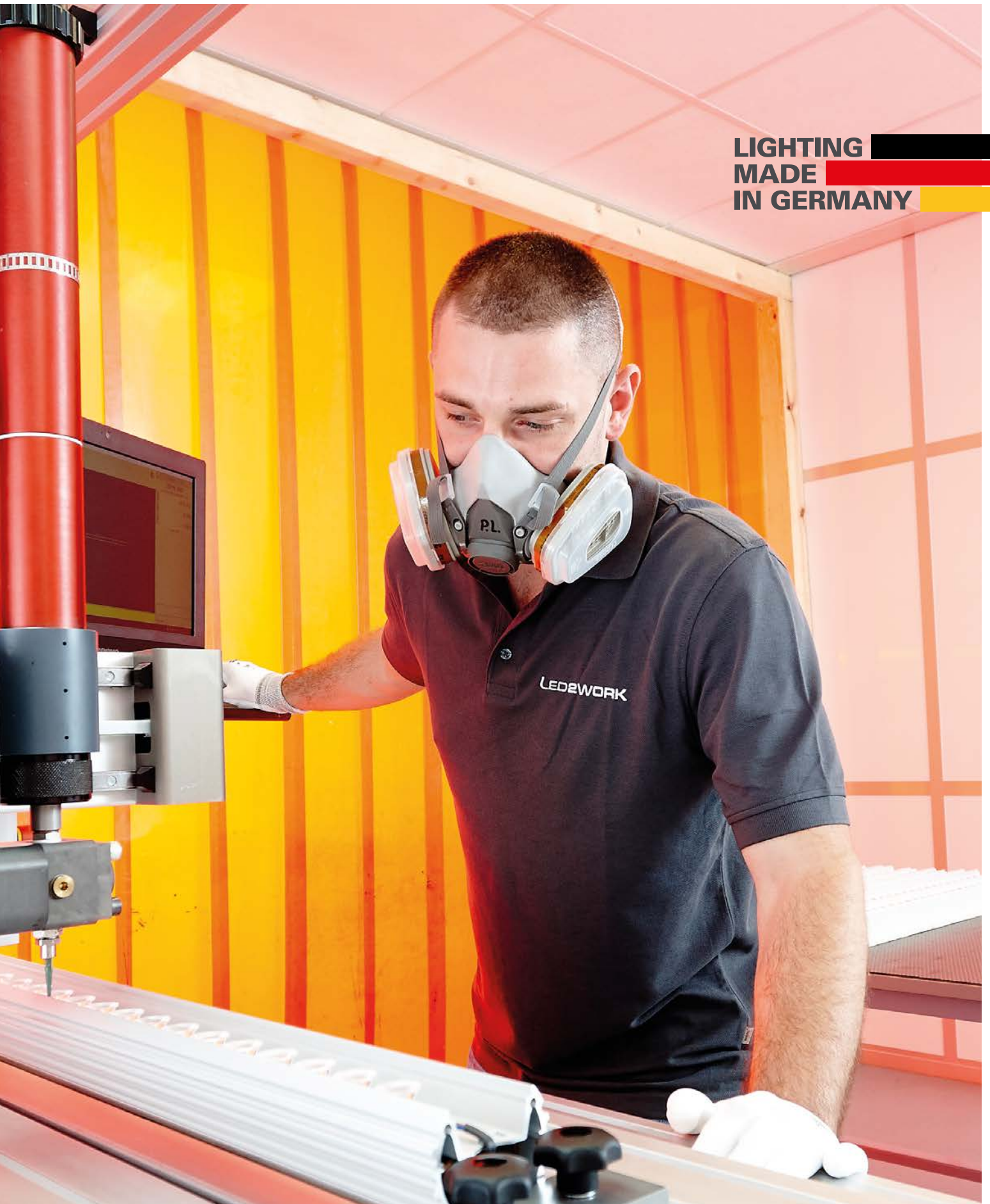
MADE IN GERMANY luminaire production: Employees setting up a CNC-controlled gluing robot
