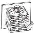
\*Mount the product on the panel, fasten bracket by pushing with tools as shown above. (In case of TC4Y, fasten bolts for bracket.)
