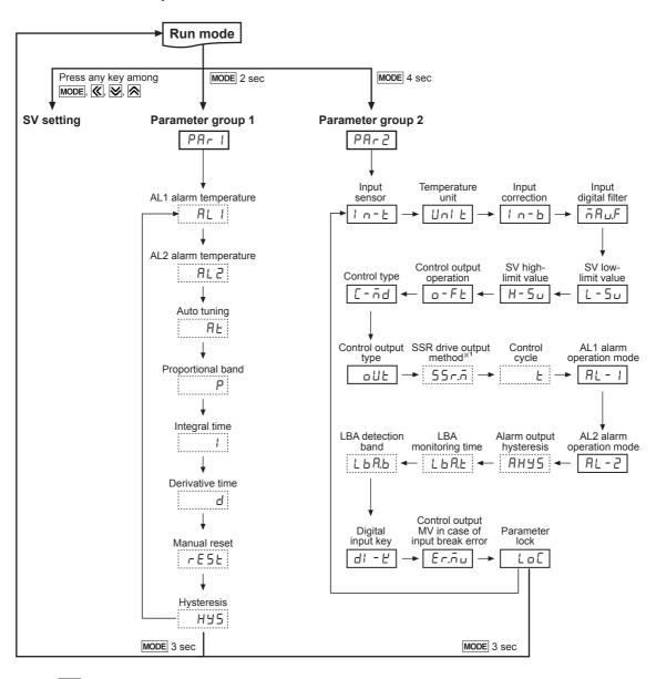
※Press MODE key over 3 sec in any setting group, it saves the set value and returns to RUN mode. (Press MODE key once in SV setting, it returns to RUN mode).
