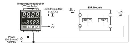
\*When selecting phase or cycle control mode, the power supply for load and temperature controller must be the same.
