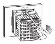
\*Mount the product on the panel, fasten bracket by pushing with tools as shown above.
