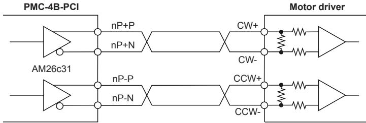
※ It is recommended to use twisted pair shield wire for pulse output signal of driver operation regarding EMC.
