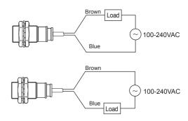
XThe load can be connected to either wire.
