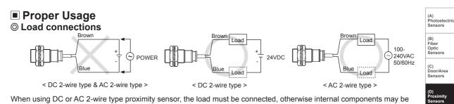
When using DC or AC 2-wire type proximity sensor, the load must be connected, otherwise internal components may be damaged. The load can be connected to either wire.
