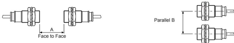
When sensors are mounted on metallic panel, it must be prevented sensors from being affected by any metallic object except target. Therefore, be sure to provide a minimum distance as below chart indicates.
