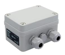
**Non-hermetic junction box NB** is used for termination of a cable with compensation tube and electrical connection to supply cable. The connection is provided using a terminal block inside the box. The junction box contains a membrane for ingress of atmospheric pressure and protection against ingress of moisture. The NB box is primarily intended for connection of hydrostatic level meters HLM-25C, HLM-25S, HLM-16N, HLM-35C and HLM-35S.
