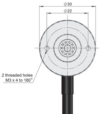
Drawing shaft type 1, connection type 1/2
