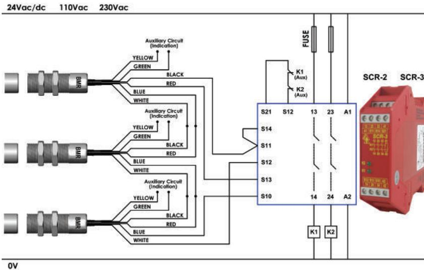
Three switches connected in series to an SCR-2 or SCR-3 to give Dual Channel guard monitoring with Automatic Start and Contactor Feedback Check.
